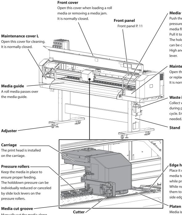
Manually cut the media along the groove.
