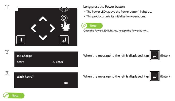
If you need to perform a head cleaning and "Wash retry? No" is displayed, tap the key to change the display to "Wash retry? Yes" and tap [Enter]. After that, follow the instructions displayed on the front panel.
