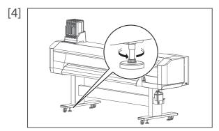
Loosen the four adjusters of Stand as shown in the left.
