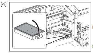
Pull the tab up of the absorption material for the flushing box, and release the hook.
