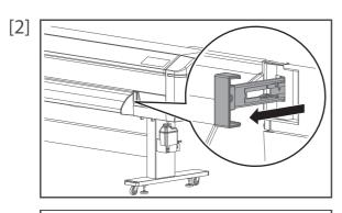
From the front side of the printer, pull the media feed lever towards you as much as possible to release the pressure rollers.
