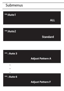
Perform automatic adjustment for all patterns (A to F) using the color sensor.
