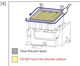
Use the cleaning stick to clean around the rubber part of the capping unit to remove the ink deposits and dust. (Capping unit) 2
