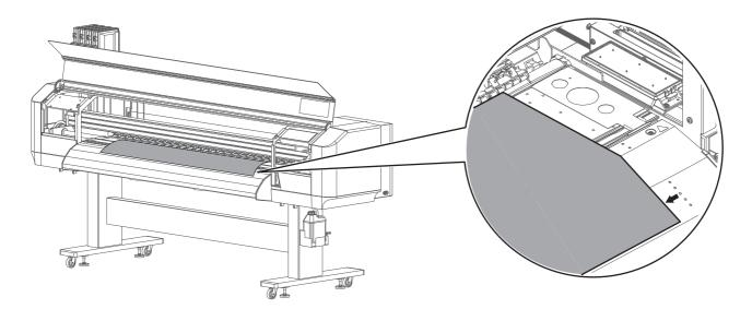
[8] If needed, use a slide lock lever on the pressure rollers to individually cancel or reduce the holddown pressure.
