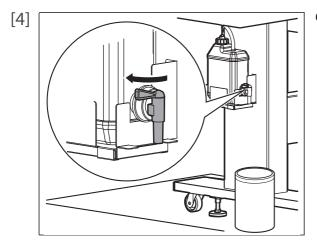
Once you empty the tank, close the waste ink valve securely. • Wipe the opening of the valve with a cloth.
