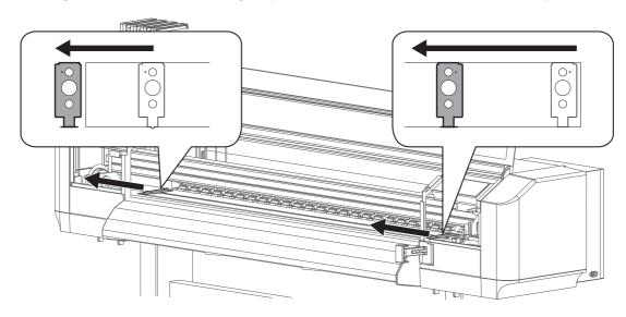
[3] Swap left and right edge holders and attach them to the platen.Insert the edge holders from the side of maintenance cover L and fit them to the groove on the platen to attach.
