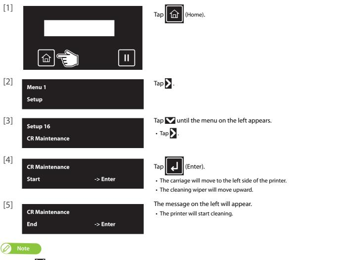
If you tap the Key while "CR Maintenance End -> Enter" is displayed, the pump is activated, sucking up the ink in the cap.
